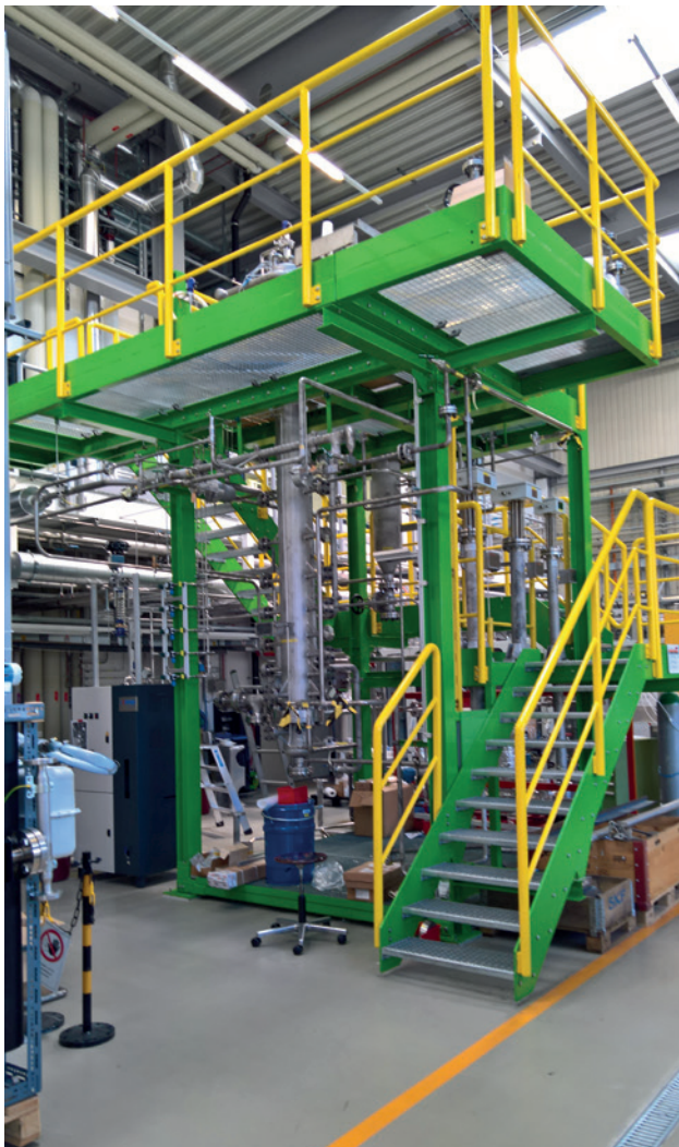
Figure 12: SCCER BIOSWEET pilot plant (TRL 6) used to study the effects of pressure (up to 10 bar), gas velocities and particle size on the available mass transfer area in the fluidized bed methanation reactor (Photo: PSI). This knowledge can be used to improve the models used for reactor optimization and process simulations. The reactor simulations will be validated by experiments in this plant.
